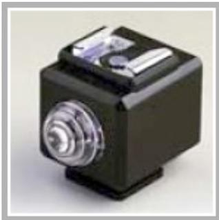
This approach is the only option available for people whose cameras don’t have hot-shoes. What happens is that you set your camera to fire its flash. A photoreceptor in your off-camera flash (this flash is called the “slave” flash) detects the camera’s flash and fires the slave.
